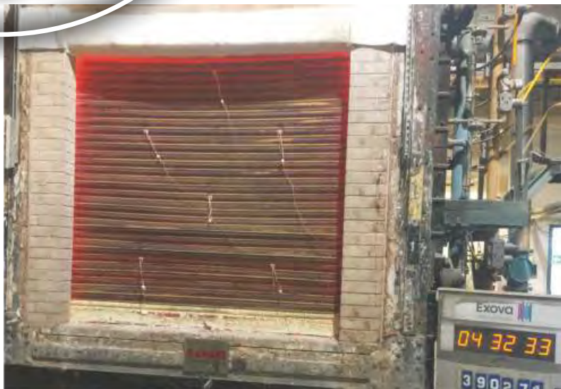
270 minutes of test - end of test
