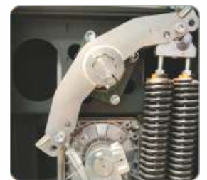
Reinforced balance system & geared motor
